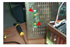
4. Remove the two screws on the Inverter Board and replace the board.
