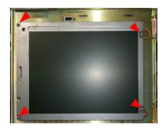
Remove the four screws holding the LCD screen in place. The LCD screen does not need to be disconnected.
